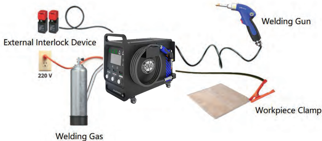
Figure 4-1 Typical Setup of the Welding System
