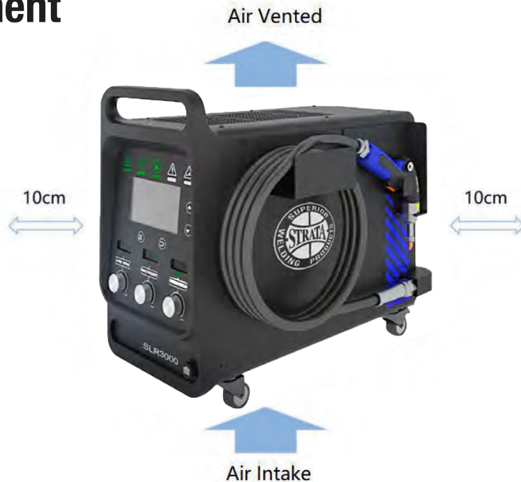
Figure 4-2 Airflow Direction and Setup Space
